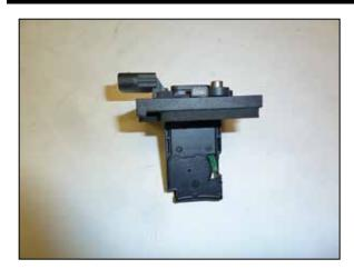
21. Install the provided gasket onto the K&N® mass air adapter. Remove the mass air sensor from the factory housing and install it into the mass air adapter and secure with the provided hardware.
