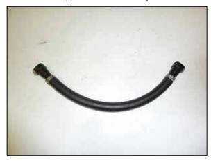
24. Install the provided quick connect fittings into the provided crank case vent hose and secure the provided hose clamps.
