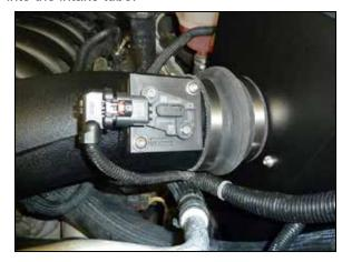
26. Connect the mass air sensor electrical connection.
