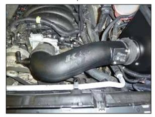
23. Install the intake tube into the coupler at the filter adapter and then into the coupler at the throttle body, adjust the tube for best fit and then secure with the provided hose clamps.
