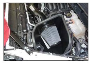
26. Install the  $K\&N^{\otimes}$  air filter onto the adapter and secure with the provided hose clamp.
