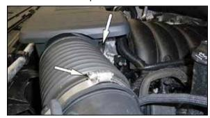
4. Loosen the hose clamps that secures the intake plenum to the air filter housing and to the throttle body. Disconnect the plenum connections at the air filter housing and then rotate the plenum counter clockwise to disengage the keyed mount and separate it from the throttle body.
