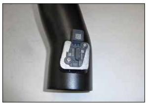
21. Remove the mass air sensor from the factory housing. Install the mass air sensor into the K&N® intake tube and secure with the provided hardware.
