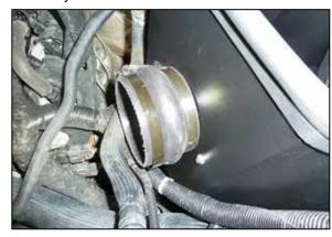
18. Install the provided hump coupler onto the filter adapter and secure with the provided hose clamp.
