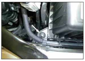
9. Remove the nut that secures the air filter housing. Unhook the wiring harness from the filter housing and then remove the air filter housing from the vehicle.
