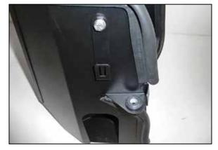
12. Install the provided wiring connector mounting bracket onto the heat shield using the provided hardware. Install the factory mounting grommet into the heat shield as shown.
