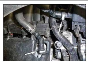
3. Depress the locking tabs and then disconnect the crank case vent line from the intake plenum and valve cover vent port.
