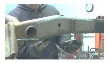
You can clamp your part into place with c-clamps to ensure a tight fit.
