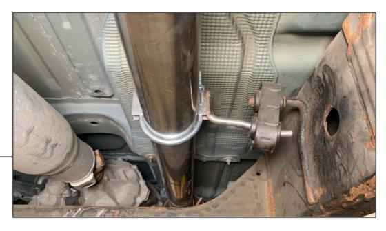
Support the front pipe and muffler using the clamp on hanger.
