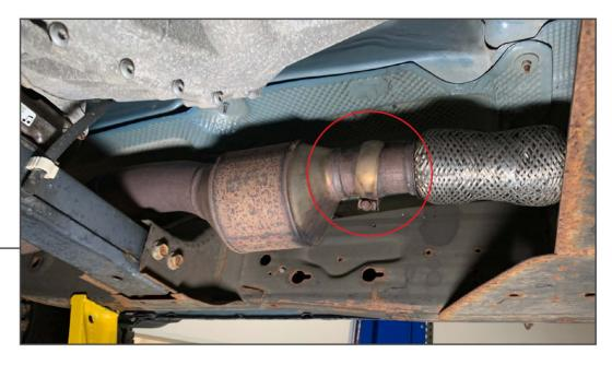
Begin by raising and supporting the vehicle with a jack and jack stands to gain better access to the factory exhaust system. Locate right in front of the joint. Using a 13mm socket loosen the clamp. Then slide it forward and away from the tail pipe.
