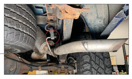
Locate and remove the rear most exhaust hanger from the tailpipe.
