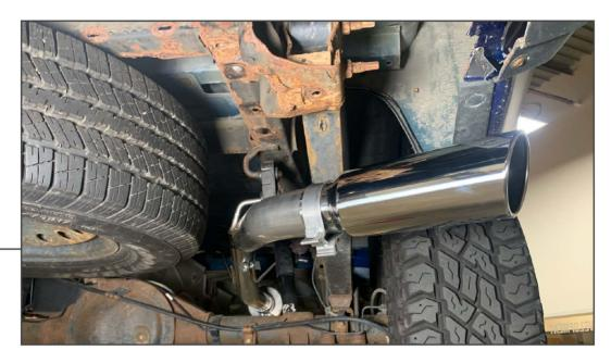
Slide (1) exhaust clamp onto the side exhaust pipe. Install the pipe onto the rear muffler pipe and into the factory exhaust hanger. Install the exhaust tip using (1) exhaust clamp.
