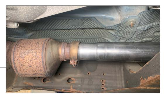
Loosely install the front pipe to the factory exhaust using the factory clamp. If your application requires the use of the mid pipe, install the mid pipe to the front pipe using (1) of the provided exhaust clamps.
