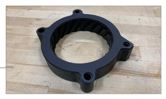
Place the supplied gasket on the throttle body (T.B.) Side of the spacer. Line the spacer up to the back of the throttle body.
