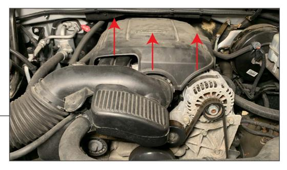
Firmly pull up on the front edge of the engine cover to remove it from its mounting post. Then set the cover aside for reinstallation later.
