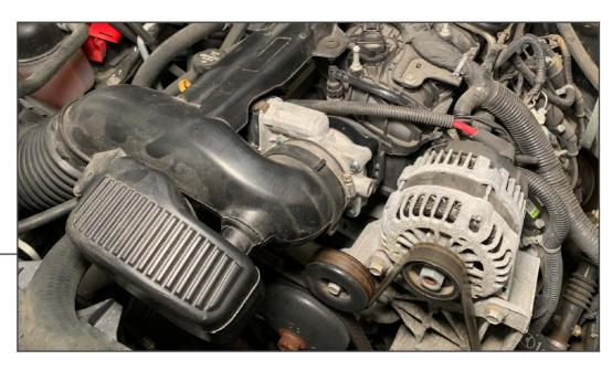
Install the throttle body and spacer assembly to the intake manifold using the provided washers and 75mm Hex head bolts. Torque to 7.5 ft-lbs. Reinstall the air intake housing in reverse order to complete the installation.
