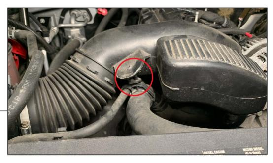
Using a panel removal tool, remove the clip securing the upper radiator hose to the air intake housing.
