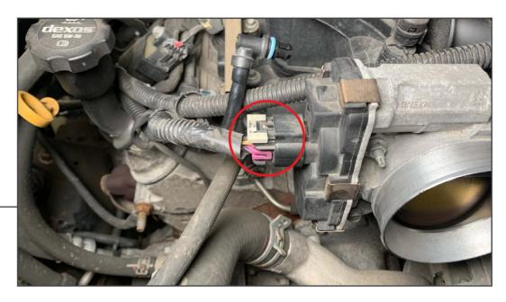
Slide back the gray locking tab from the throttle body electrical connection. Depress the tab while pulling the plug away from the throttle body. Loosen and remove the (4) 10mm fasteners securing the throttle body to the intake manifold. Remove the throttle body from the vehicle.
