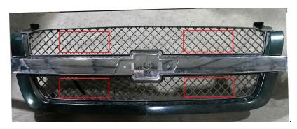
(2) Open the package, take out the studs, and place each stud into the welded nut on the mesh grille frame, see below. (Some grille will come with bolt welded directly to the grille frame.)
