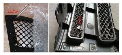
(3) Install the mesh grille into the grille opening. Place the washer and nut on the stud, loosely tighten the nut. Center the grille in the opening. Adjust the light as needed. Then tighten the remaining hardware.
