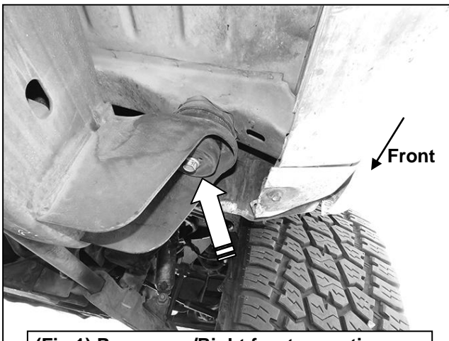
(Fig 1) Passenger/Right front mounting location. Temporarily remove the body bolt
