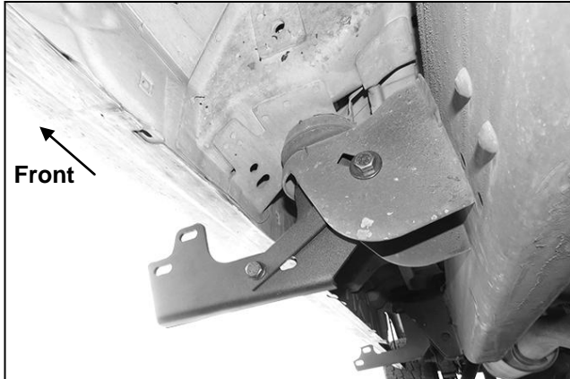
(Fig 12) (1) Center Support Bracket attached to the body mount and Mounting Bracket
