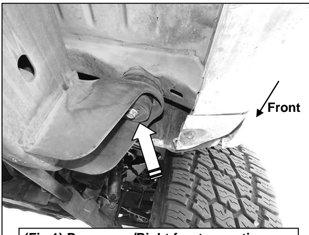
(Fig 1) Passenger/Right front mounting location. Temporarily remove the body bolt
