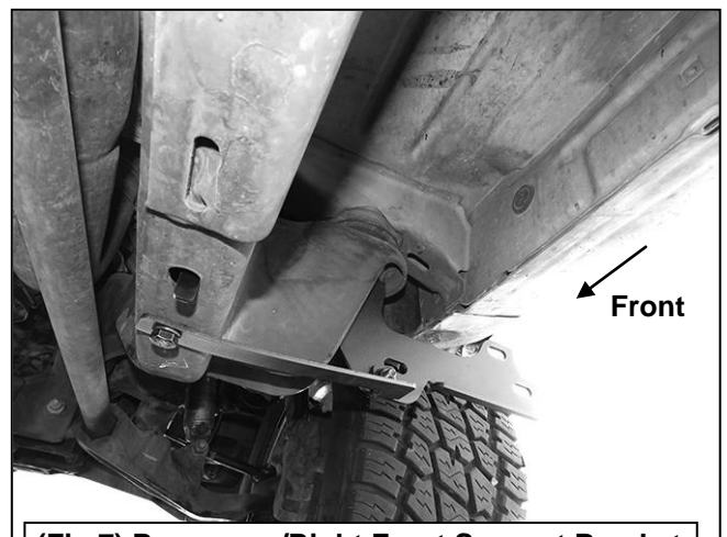
(Fig 7) Passenger/Right Front Support Bracket attached to the frame and Mounting Bracket
