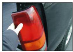
Once the screws are removed, you will be able to pull tail lens straight out.
