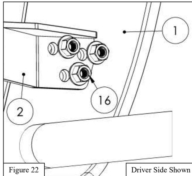
24. Adjust the grille guard as desired. Tighten and torque all hardware as specified: M10 to 32 ft-lbs. and M12 to 55 ft-lbs.
