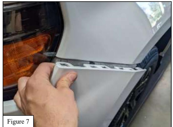
11. Remove the plastic clips holding the air intake splash shield in place, and remove the splash shield.
