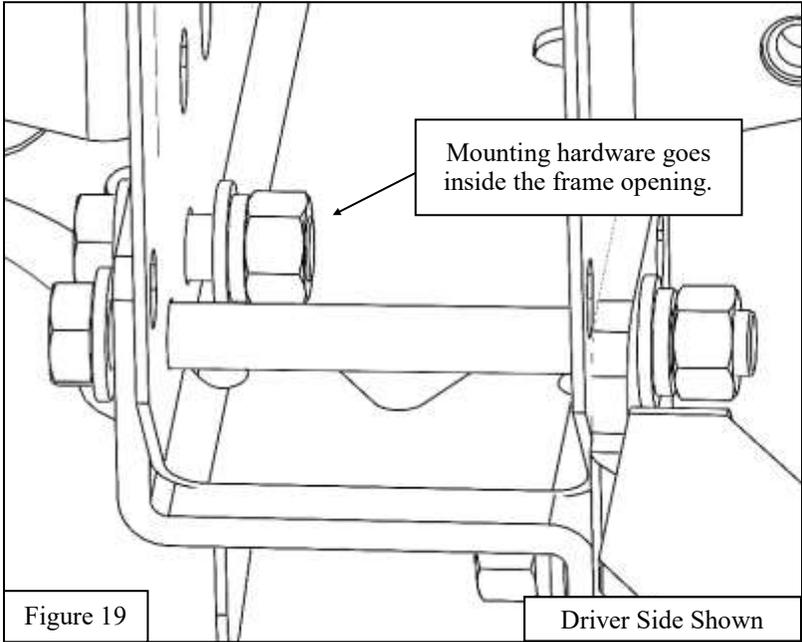
23. Use the supplied M10 (Items 12-14) and M12 Hardware (Items 15-17) to secure the grille guard assembly to the previously installed mounting brackets. See **Figures 20 through 22** for reference.
