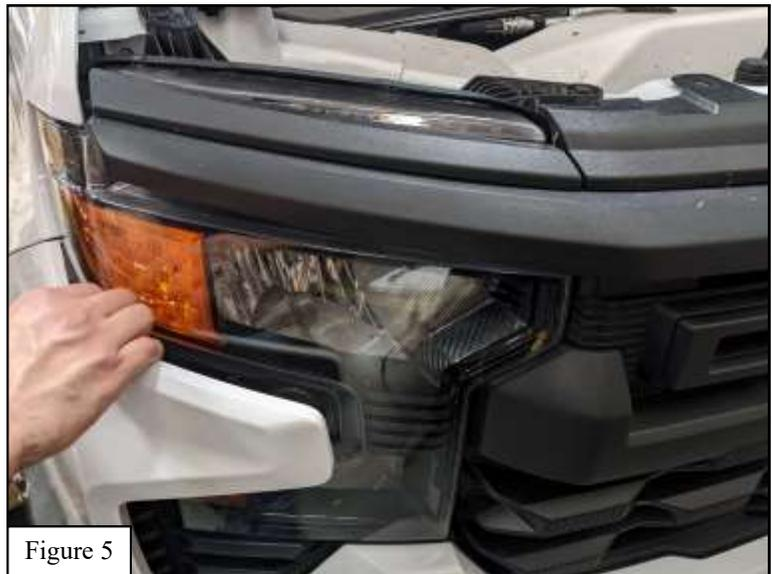
9. On both sides of the vehicle, use a pry tool to remove the fascia panel from the clips shown. See **Figures 6 & 7** for reference.
