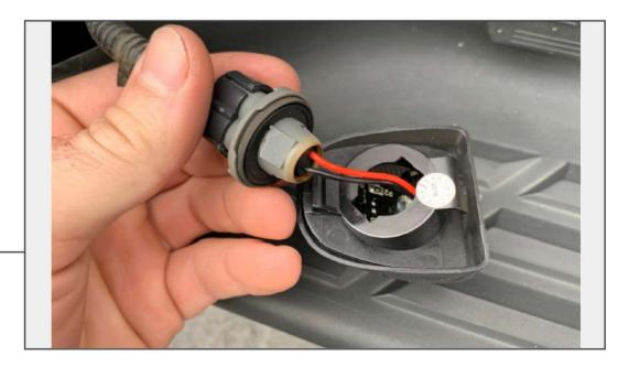
Plug the LED license plate lamp into the vehicle light socket.
