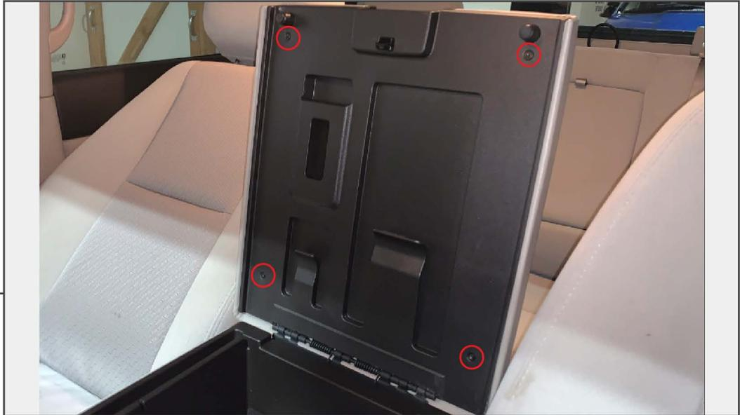
Open the center console lid. Remove (4) T-20 Torx screws. Starting from the bottom, remove the plastic panel from the center console lid.
