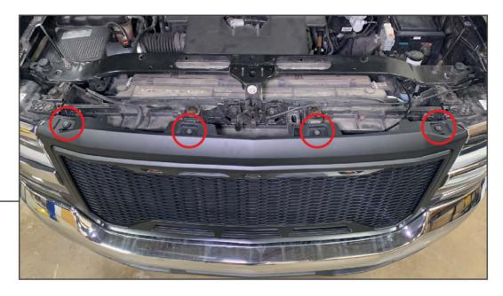
Install the upper portion of the grille to the radiator support re-using the original (4) 10mm bolts.
