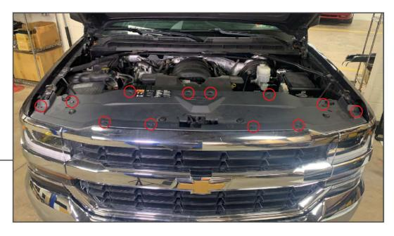
Remove the (12) plastic push clips from the radiator support cover. Remove the radiator support cover from the vehicle.
