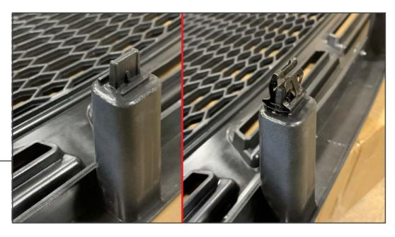
Prepare the grille for installation. Using the provided (6) metal clips, secure the clips to the mounting points on the grille.
