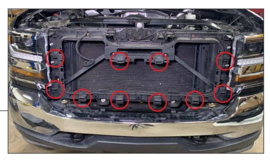
Remove the grille from the vehicle by evenly dislodging the metal clips around the grille.
