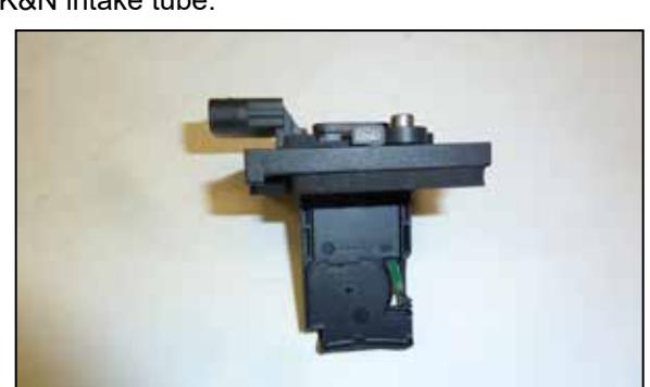
23. Remove the mass air sensor from the factory housing and then install the sensor into the adapter provided along with the gasket.
