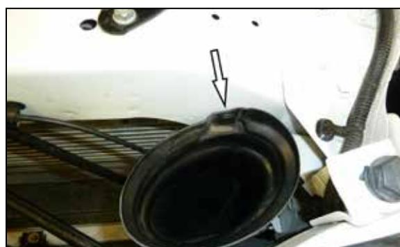
18. Install the fresh air intake duct into the K&N air filter housing and then secure it to the core support using the factory push pin.
