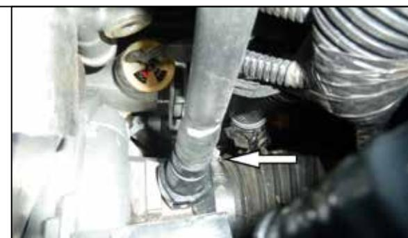
5. Loosen the hose clamp that secures intake tube to the turbo inlet.
