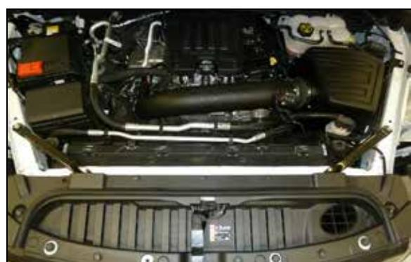
34. Reinstall the upper radiator valence and secure with the ten factory push pins.
