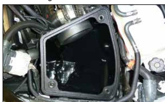
17. Install the K&N air filter housing into the vehicle and secure with the factory nut from step #12.
