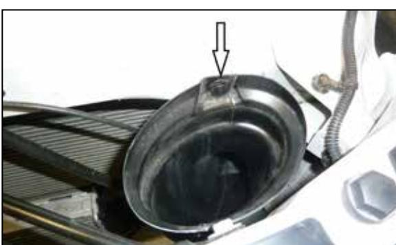
10. Remove the push pin that secures the fresh air duct to the core support and then dislodge the duct from the air filter housing. This push pin will be reused in a later step.
