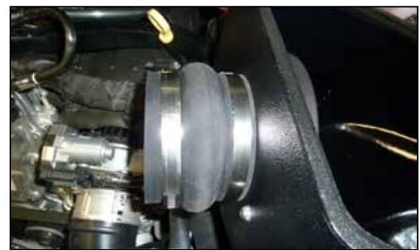
20. Install the hump coupler onto the filter adapter and secure with the provided hose clamp.
