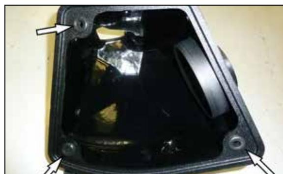
16. Install the three provided grommets into the K&N air filter housing as shown.
