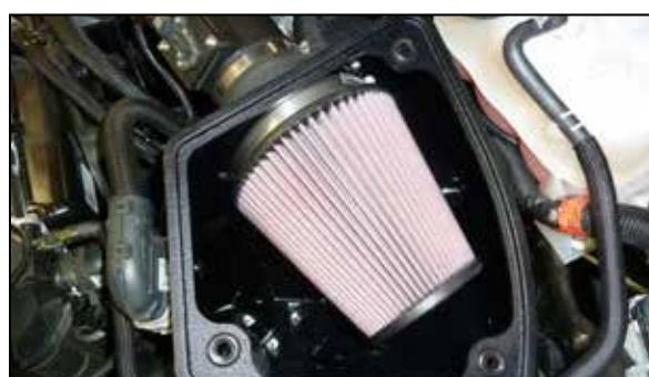
32. Install the K&N air filter onto the filter adapter and secure with the provided hose clamp.
