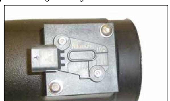
24. Install the mass air sensor assembly into the K&N intake tube and secure with the provided hardware as shown in the photo.
