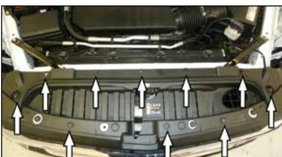
9. Remove the ten push pins that secure the upper radiator valence and then remove the valence from the vehicle.
