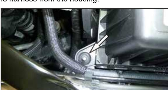
12. Remove the nut that secures the air filter housing to the mounting bracket. This nut will be reused in a later step. **NOTE: K&N Engineering, Inc., recommends that customers do not discard factory air intake.**
