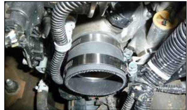
21. Install the provided straight coupler onto the turbo inlet and secure with the provided hose clamp.
