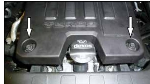
6. Remove the two bolts that secure the engine cover to the engine and then remove the cover from the vehicle. These bolts will be reused in a later step.
