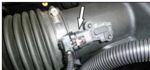
2. Disconnect the mass air sensor electrical connection and loosen the hose clamp that secures the factory intake tube to the air filter housing.
