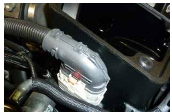
19. Install the wiring harness bulk connector onto the bracket installed onto the K&N air filter housing.
