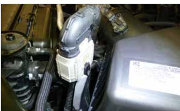
11. Using a small pick or similar tool, release the locking tab that secures the wiring harness bulk connector to the air filter housing and then remove the harness from the housing.
