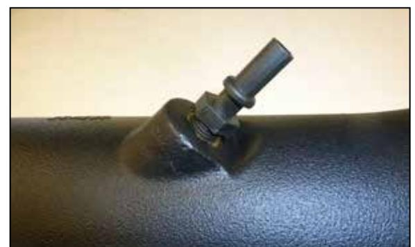
22. Install the provided quick connect fitting into the K&N intake tube.
