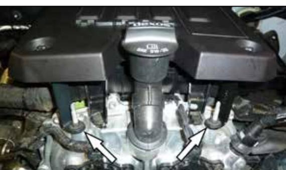
28. Install the engine cover onto the engine and secure the brackets to the factory mounting studs using the factory nuts.
