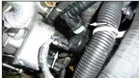
4. Depress the locking tap and then disconnect the CCV pipe from the solenoid attached to the factory intake tube. Disconnect the solenoid electrical connection.
