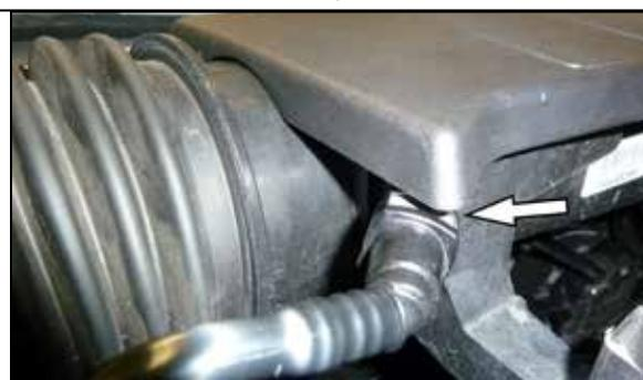
3. Depress the locking tab and then disconnect the CCV pipe from the plenum.
