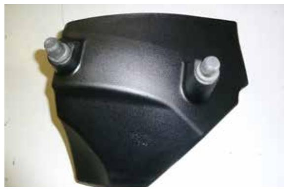
15. Remove both factory air filter housing bushings from the factory housing and install them onto the K&N filter housing as shown.
