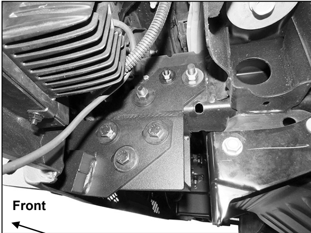
(Fig 23) Driver/left side of Bumper attached to Frame Bracket (Note cube light installation)
