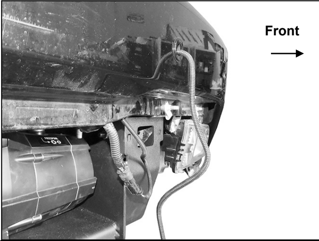
(Fig 21) Reinstall factory bumper. Models with sensors, plug Wire Harness Extensions into the sensors in the HD Bumper
