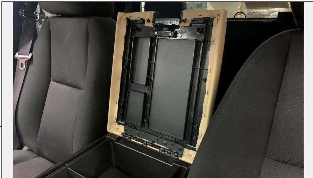
Install the new center console lid to the vehicle re-using the original (4) Phillips head screws. Tighten until secure, do not over-tighten.
