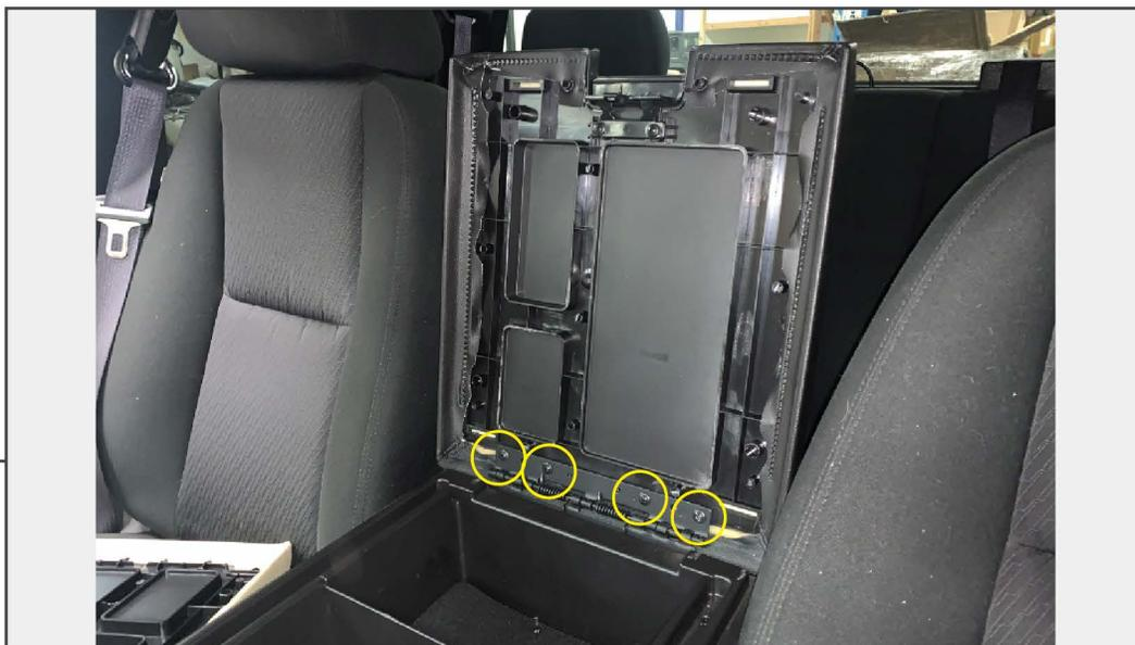
Remove (4) Phillips screws from the hinge going through the center console lid. Remove the lid from the vehicle.
