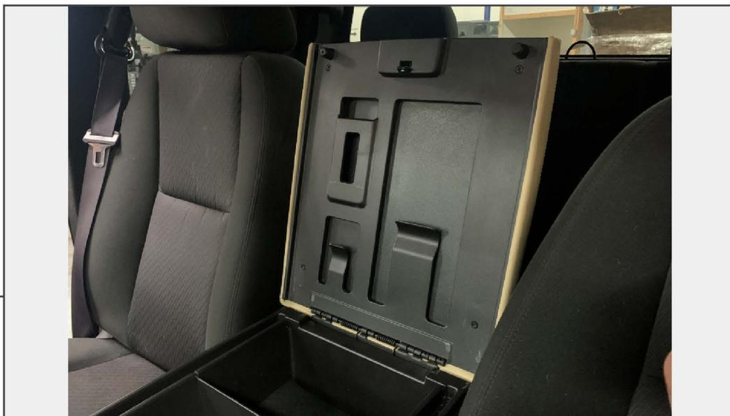
Install the original plastic panel to the new center console lid re-using the original (4) T-20 Torx screws. Tighten until secure, do not over-tighten.
