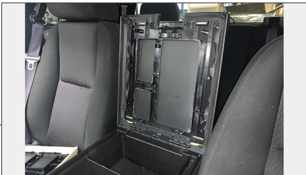
Using a plastic panel pry tool, remove the plastic panel from the center console lid.
