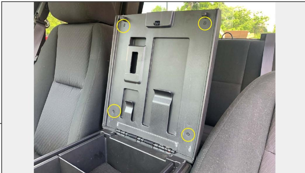
Open the center console lid. Remove (4) T-20 Torx screws from the plastic panel on the lid.
