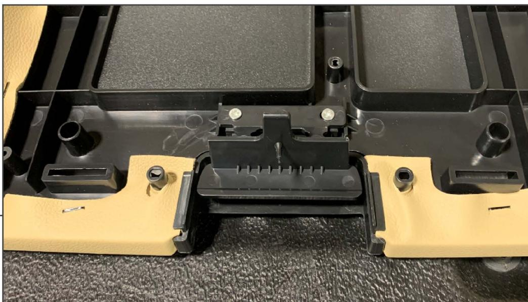
Remove the (2) pre-installed Phillips screws in the new center console lid, then install the provided center console latch into the lid. Tighten the screws until secure, do not over tighten.
