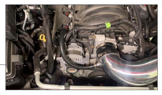
Use the (1) provided PCV hose and (2) 1" hose clamps to attach the PCV on the engine valve cover to the intake tube. Cut the hose to best fit if necessary and tighten the clamps to secure into place.
