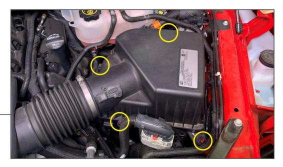
Remove (4) 10mm bolts from the air box lid. Remove (1) 10mm nut from the lower air box.
