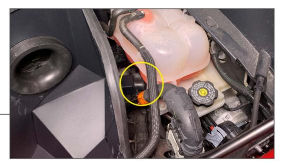
Use (1) M6 locking nut and (1) M6 flat washer (25mm OD) to secure the heat shield to the bracket below the coolant reservoir.
