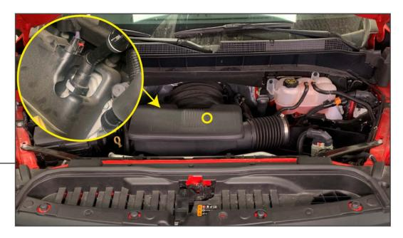
Loosen (1) hose clamp attaching the air intake tube to the throttle body. Unplug the PCV hose from the intake tube and the valve cover by pressing the gray tab inward while pulling the hose outward. Remove the intake tube from the vehicle.
