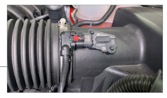
Unplug the MAF sensor from the intake. Slide the red tab outward, then press the black tab while pulling the connector from the sensor.
