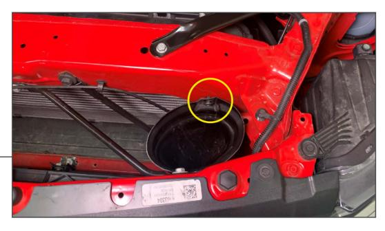
Re-install the air routing tube to the vehicle using the (1) original push clip.
