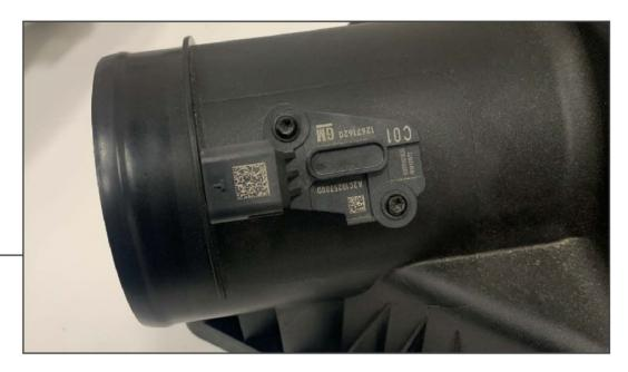
Remove (2) T-20 Torx screws from the MAF sensor to remove the sensor from the original intake housing.
