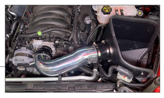
Install the intake tube to the air filter adapter using (1) 4" coupler and (2) 4" hose clamps. Install the intake tube to the throttle body using the appropriate coupler and clamps (see note below).
