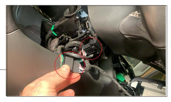
Locate the flat plug at the base of the steering wheel. Unplug it and install the supplied T-harness. Route the other end of the T-harness to the navigation unit. Then re-assemble the steering column and dash panels in reverse order.
