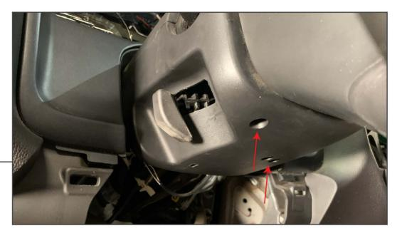
If applicable, remove the screws securing the steering wheel trim together. Then using a soft pry tool, separate the two halves.
