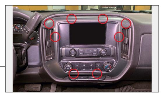
Using a soft pry tool, pry around the radio bezel to release the (8) clips.
