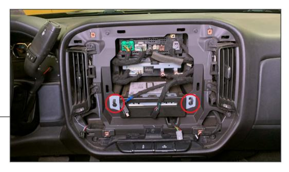
Remove (2) screws on the CD player. Remove the CD player from the dashboard and unplug the electrical connector. The CD player will not be reused.
