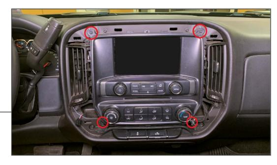
Using a 7mm socket, remove the (4) screws securing the original radio to the dashboard.
