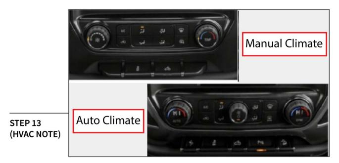
Identify the vehicle's HVAC unit, see photo above. Once the navigation unit is installed, use the directory below to select the vehicle HVAC system to ensure proper HVAC function.
