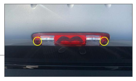
Remove (2) T-20 Torx screws from the third brake light housing.
