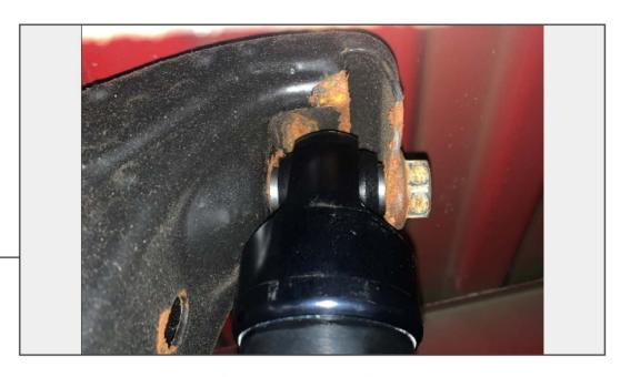
Install the new shock absorber to the vehicle frame using original hardware.
