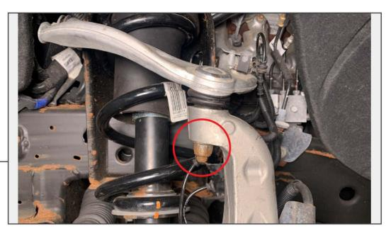
Loosen (1) 21mm nut on the upper ball joint. Once loose, strike the knuckle with a hammer to dislodge the ball joint from the knuckle. Once dislodged, remove nut from ball joint.
