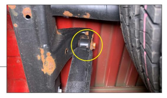
Remove (1) 21mm bolt from the top of the shock absorber.
