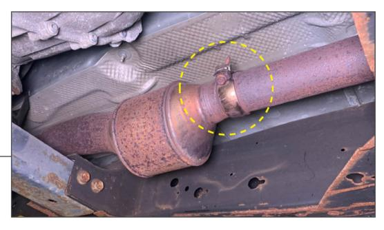
Loosen (1) exhaust clamp at the catalytic converter. Loosen enough to release tension from the ball flange.
