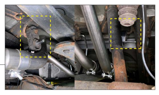
Install the (1) RH over axle pipe into the original vehicle rubber exhaust hangers. Insert the pipe into the muffler and loosely secure using (1) 2.5" exhaust clamp.
