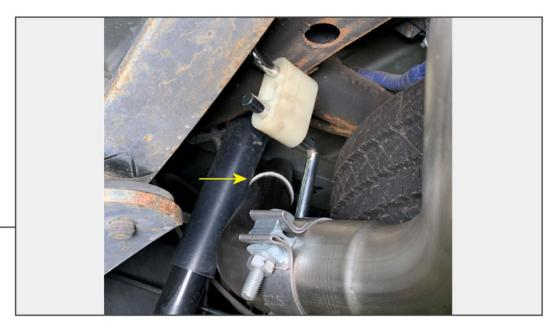
Install (1) plastic exhaust hanger onto the 'L' bracket. Install the (1) LH tail pipe into the previously installed over axle pipe. Install the tail pipe into the exhaust hanger previously bolted to the frame. Loosely secure the pipes using (1) 2.5" exhaust clamp.
