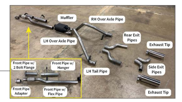
Lay out and identify all exhaust components.
