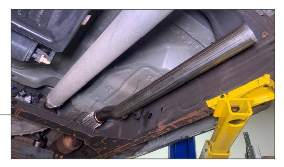
**07-08 Models:** Install the (1) front pipe w/ flex pipe into the vehicle, then install (1) exhaust clamp w/ hanger onto the front pipe and insert into the vehicle rubber hanger along the frame. \*The front pipe welded hanger will not be used.
