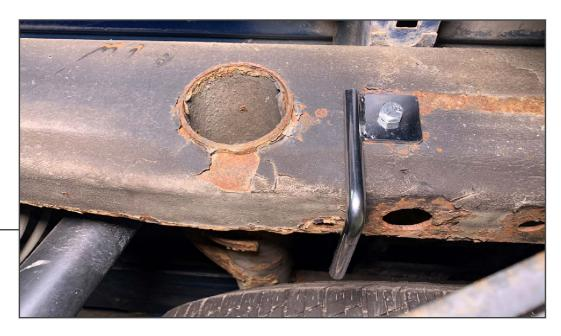
Install the supplied exhaust hanger bracket to the vehicle frame using the provided (1) M10x1.50  $\times$  40mm bolt, flat washer, lock washer, and hex nut. Torque to 25 ft.-lbs.
