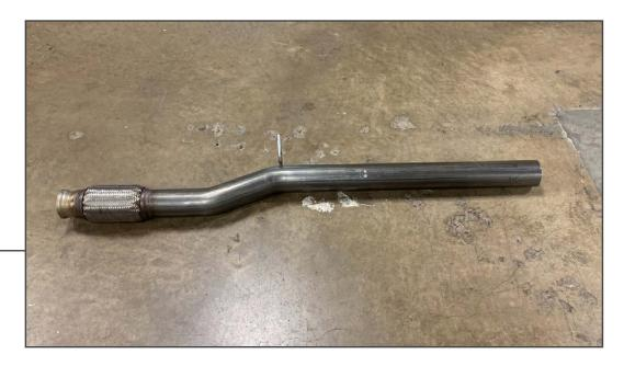
Depending on vehicle cab/bed configuration, trimming the front/mid pipe may be necessary.
