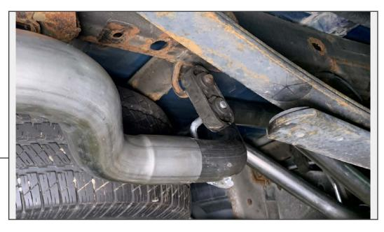
Hang the right side exhaust pipe to the original rubber exhaust hanger.
