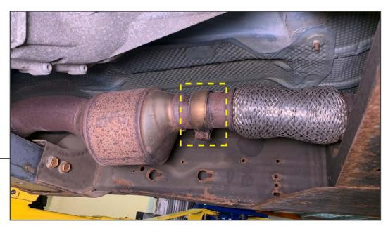
Lift and support the vehicle to gain access to the factory exhaust system. Locate the (1) exhaust clamp after the catalytic converter. Use a 13mm socket to loosen the exhaust clamp.
