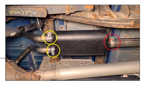
Install the right and left side pipes into the original vehicle rubber exhaust hangers. Align the muffler in between the front and side pipes. Loosely secure the muffler using (2) 2.5" exhaust clamps, and (1) 3" exhaust clamps.
