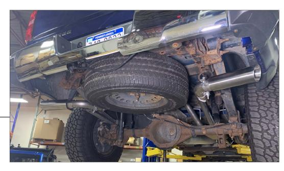
With the exhaust loosely installed, finalize adjustments and tighten all of the exhaust clamps. Work from the front of the vehicle to the exhaust tips. Rotate the muffler/pipes as need for best fit. Tighten the exhaust clamps to 45 ft.-lbs.
