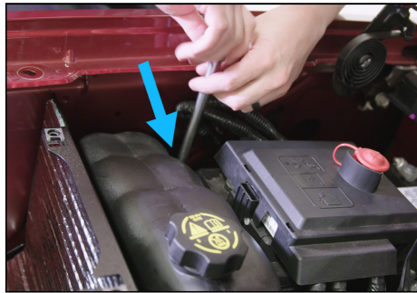
21. Reinstall the coolant reservoir.
