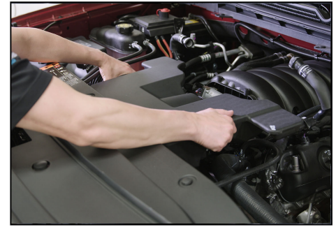
6. Remove CLEAN/AIR DUCT RESONATOR from vehicle.
