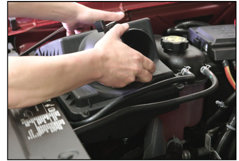
9. Remove OEM AIR INDUCTION HOUSING.
