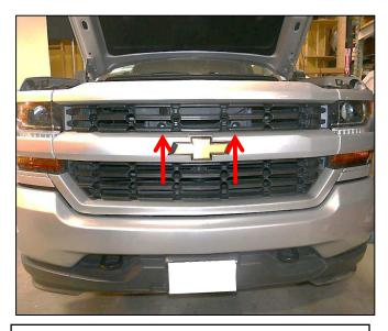
Step 3 Looking toward the vehicle locate and remove 2 factory hex head bolt using a 10mm socket as shown. Discard factory hardware.
