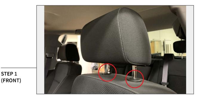
Clean the vehicle seats using a vacuum cleaner. Remove the front seat head rest by pressing the (2) buttons at the headrest base.
