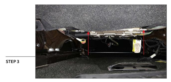
Behind the front seat, disconnect the (2) plastic clips attached to the elastic bands to allow the rear felt panel to release from the seat. Allow the panel to hang loose, the panel will be flipped upwards when installing the seat cover.
