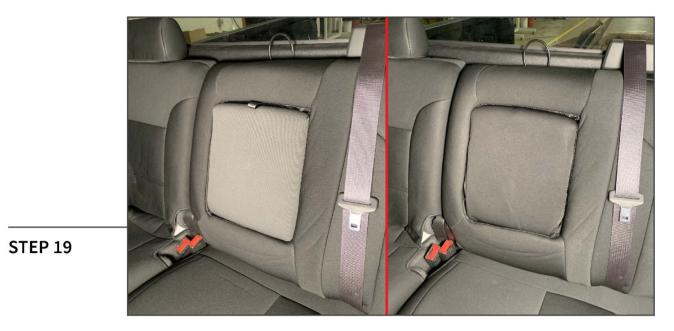
Ensure the center armrest area of the backrest seat cover is properly tucked into the plastic trim area of the armrest cutout. Install the rear arm rest cover to the seat.
