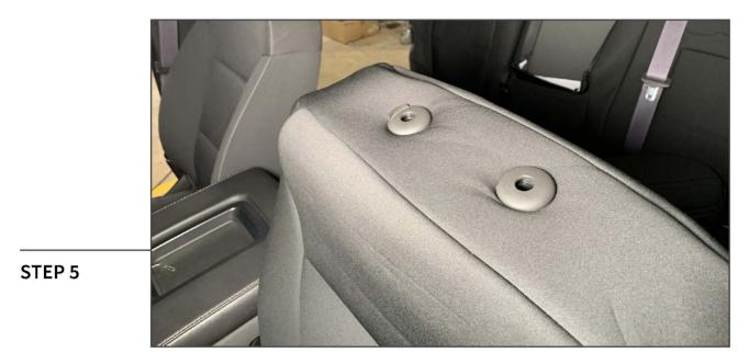
Tuck the (2) headrest holes in the cover under the (2) headrest mounting points on the seat.
