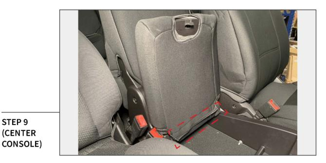
Open the middle seat base storage area, and slide the cover onto the seat base storage area lid. Secure the cover using the attached Velcro along the bottom.
