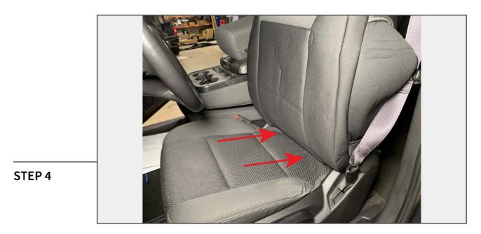
Drape the front seat cover over the front seat, ensuring the airbag cutout is facing out and the rear panel is flipped upwards. Route the Velcro in between the upper and lower seat cushion.
