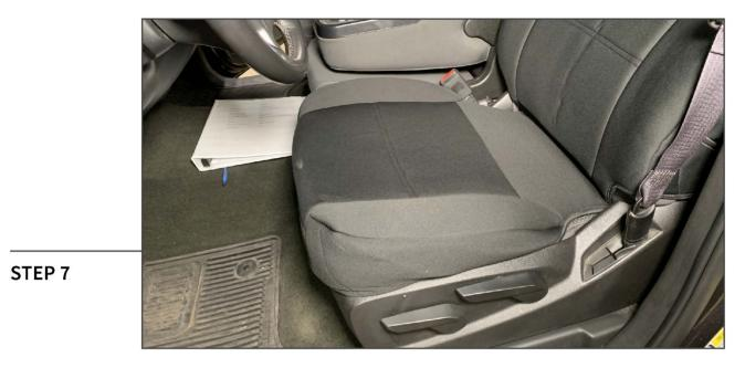
Place the front base cover to the front seat and tuck the (2) rear straps in between the backrest and the base towards the underside of the seat. Tuck the sides of the cover under the plastic trim for best fit. Latch and tighten the (2) straps under the seat, ensuring not to interfere with any under-seat components. Secure the (2) nylon straps to the sides of the seat to secure the sides.
