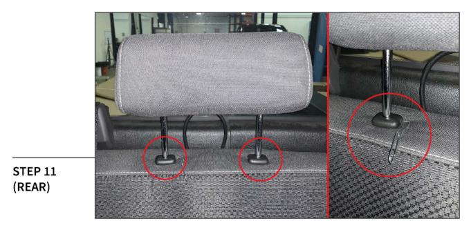
Using a pick/paperclip, press the (2) inner buttons on the headrest mount to release the headrest from the seat backrest.
