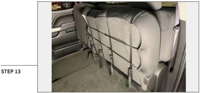
Drape the rear seat base cover over the rear seat, then fold the seat upwards to reveal the straps. Latch and tighten the (4) straps under the rear seat base. Pull and secure the (2) nylon straps to each other under the seat.
