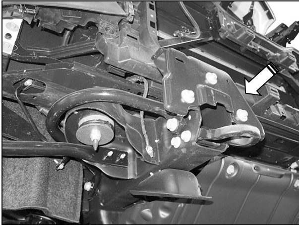
(Fig 6) Remove factory bumper brackets and tow hooks if equipped (passenger/right side pictured)
