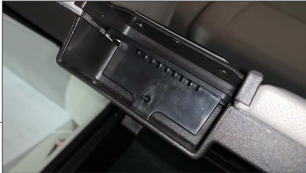
Install the new center console lid latch to the center console lid reusing original hardware. Re-install the plastic panel onto the center console lid reusing original hardware.
