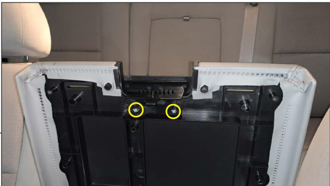
Remove (2) Phillips head screws from the center console lid latch. Remove the latch from the center console lid.
