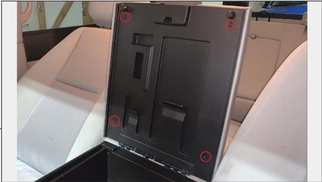
Open the center console lid. Remove (4) T-20 Torx screws. Starting from the bottom, remove the plastic panel from the center console lid.
