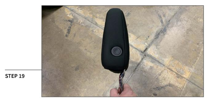
Install the headrest cover onto the rear seat headrests. Tuck the headrest cover under the tilt button. Install the headrests onto the rear seat backrest.
