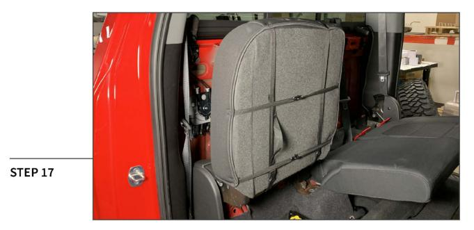
Place the seat cover onto the rear seat base, connect the (2) straps together. Make final adjustments, then tighten the straps. Hook the (2) elastic straps together to secure the sides of the seat cover.
