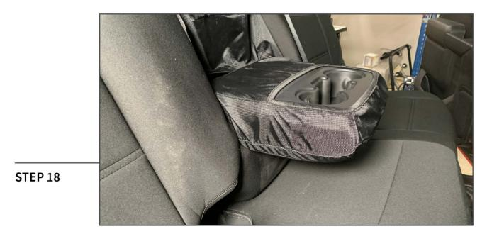
Install the rear seat backrest to the vehicle following steps 12-14 in reverse order. Pull the center armrest down, and install the armrest cover. Secure the cover using the attached Velcro.
