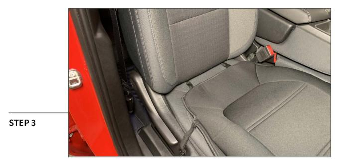
Lay the front seat cover base onto the seat, and route the (2) strap buckles in between the seat base and backrest.
