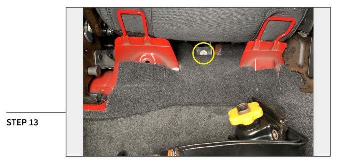
Under the seat, remove (4) silver 10mm bolts along the rear of the cab.
