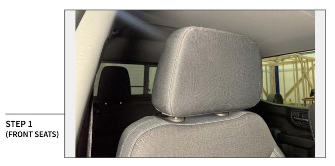
Remove the headrest from the front seat by pressing the (2) buttons at the base of the headrest. Set headrest aside.
