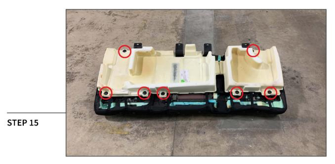
Lift and remove the rear seat backrest from the vehicle. Place the backrest on a soft surface. Using a panel removal tool, remove the (7) plastic push clips to remove the foam sound deadening from the backrest.
