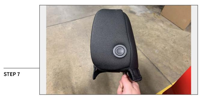
Install the headrest cover onto the vehicle headrest. Tuck the headrest cover under the tilt button.
