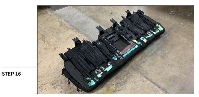
Place the seat covers onto the backrest and route the attached straps towards the back of the seat. Connect the (8) seat cover straps together. Make final adjustments and tighten the (8) straps until secure. Secure the seat cover sides to the backrest using the (6) elastic straps per side. Re-install the foam sound deadening using the original push clips.
