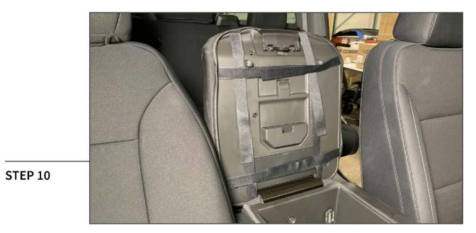
Secure the center console armrest cover using the (4) Velcro straps. Make final adjustments, and tighten the Velcro to secure into place,
