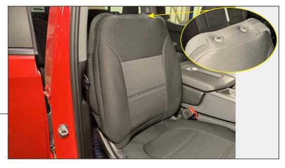
Place the front seat backrest onto the front seat. Route the attached straps between the seat backrest and seat base. Pull the seat cover downwards, and tuck the headrest base holes in the cover under the headrest base.
