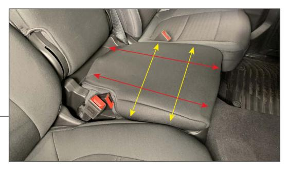
Secure the jump seat base cover using the (2) attached buckle straps and (4) elastic straps. Make final adjustments, and tighten the (2) buckle straps.
