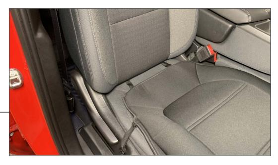
Lay the front seat cover base onto the seat, and route the (2) strap buckles in between the seat base and backrest.
