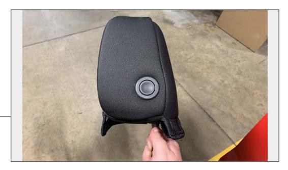
Install the headrest cover onto the vehicle headrest. Tuck the headrest cover under the tilt button.
