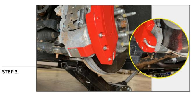
Place the lower caliper cover bracket around lower caliper bracket. Using a rubber mallet, lightly tap the caliper cover upwards to ensure proper fitment for the upper bracket.
