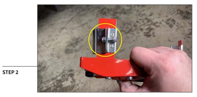
Prepare the caliper cover for installation by removing the nut and bolt from the top to separate the clamp. Set the removed bracket and hardware aside for installation later.
