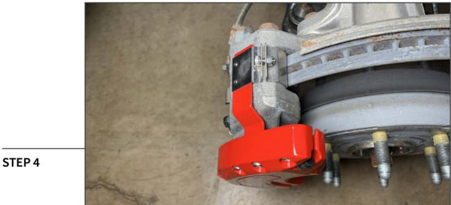
Using the previously removed bracket and hardware, secure the top of the caliper cover to the vehicle caliper bracket. Tighten the hardware until the cover is secure.
