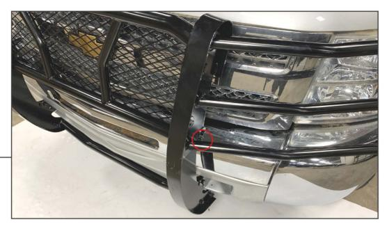
Secure the top of the grille guard to the previously installed upper brackets using (2) M8x1.25 x 25mm Allen bolts, (4) M8 flat washers - 16mm OD, and (2) M8 lock nuts per side.
