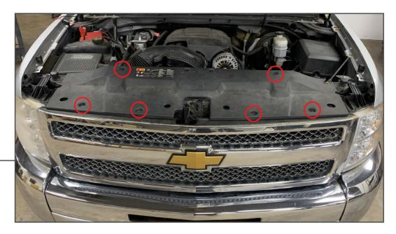
Open the vehicle hood. Remove (6) plastic push clips from the radiator cover. Remove the cover from the vehicle.
