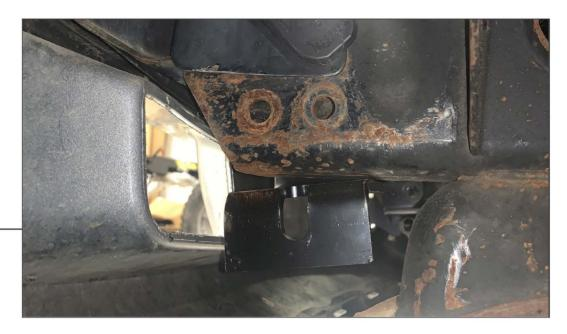
Install the (1) frame rail adapter to the vehicle frame rail using (2) M12x1.75 x 40mm bolts, (4) M12 flat washers, (2) M12 lock washers, and (2) M12 nuts.
