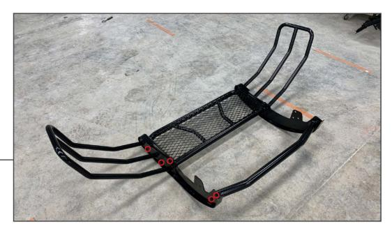
Place all brush guard components on a soft surface. Assemble the headlight guards, center grille guard, lower cross bar, and front bumper bars using (5) M8x1.25 x 25mm bolts, (10) M8 flat washers, and (5) M8 lock nuts per side.
