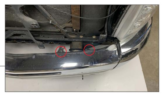
Remove (2) 15mm bolts from the top of the bumper mounting bracket.
