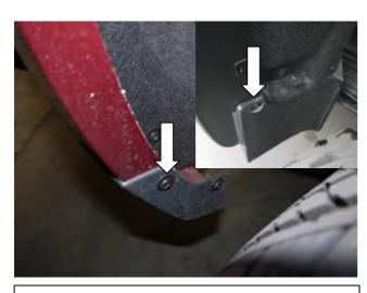
**STEP 14:** Using #15 Torx head screwdriver loosen the top wheel arch facing screw in the front aero spoil. Then remove upper screw from the rear factory mudguard. Maintain screw for re-install.
