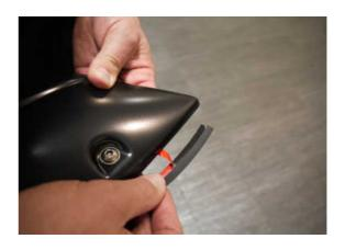
**STEP 11:** Attach the included rubber seal to the Fender Flares. Peel back 2" of the adhesive backing and position on the Fender Flare. Attach the seal to the Fender Flare, peeling back a few inches at a time. Ensure pressure is used to secure rubber seal to Fender Flare edge. Attach rubber seal along all areas the Fender Flare will make contact with the vehicle body. Trim excess rubber seal.
