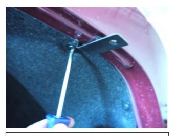
**STEP 7:** Apply clear tape to the inside edge of the fender wheel arch in front of positions **A**, **B** and **C** (step 5) over mastic sealant. Install the large brackets in positions **A**, **B** and **C** (step 5) aligning the slot in the bracket with the vacant holes from the factory screws in the vehicle wheel arch. Ensure clips are positioned over the clear tape. Re-install the factory screws in location **A**, **B** and **C** using a #15 Torx head screwdriver.
