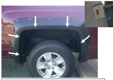
**STEP 15:** Slide the front inner edge of the fender flare behind the aero spoil where previous screw was loosened. To secure, apply upward / inward force toward the vehicle fender. Slide the black metal clips over the Fender Flare and the inner wheel arch lip in the five locations shown. Position so that the barb in the clip locates in the slot of the Fender Flare.
