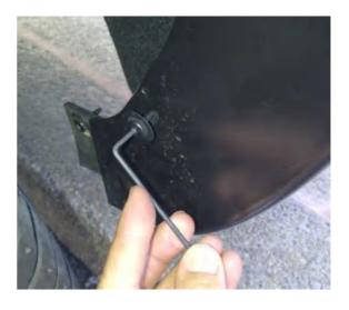
**STEP 17:** Using #15 Torx head screwdriver re-install the upper screw from the rear factory mudguard through the slot in the Fender Flare. Ensure all fixing points are tight and secure and that the rubber seal is flush neatly against the vehicle body.
