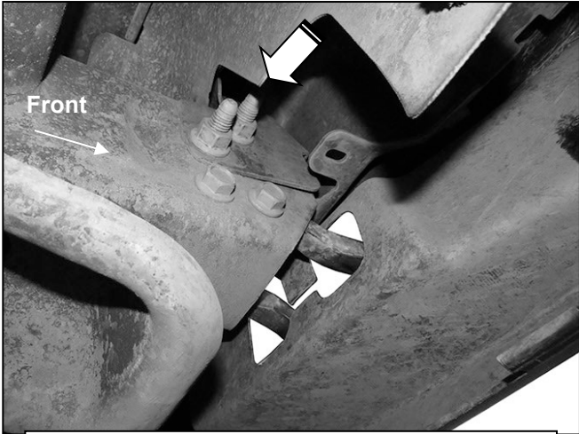
(Fig 2) From behind bumper, remove the hex nuts, (see arrow), and double bolt plates attaching the bumper bracket to the frame. Also temporarily remove the tow hooks if equipped, (Passenger/right side pictured)
