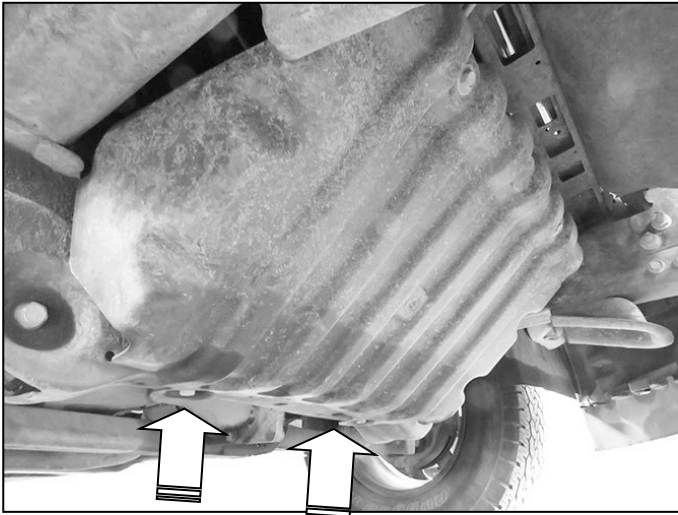
(Fig 1) Temporarily remove (2) factory bolts attaching splash guard to crossmember (arrows)
