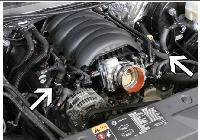
17. Install the coupler onto the throttle body along with the provided t-bolt clamps, then remove the two breather tubes from the vehicle.
