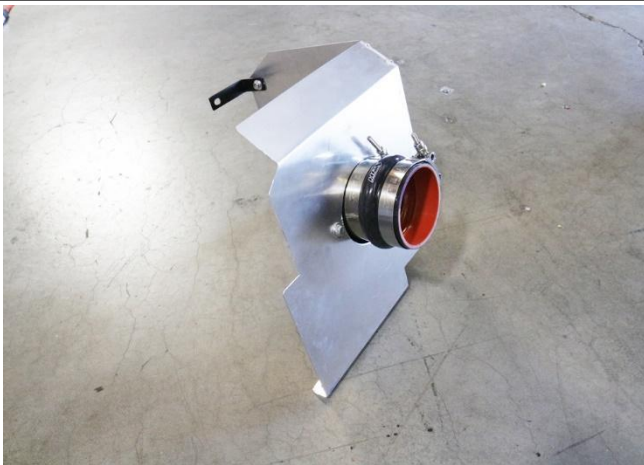
14. Install the hump coupler with the provided t-bolt clamps onto the velocity stack.
