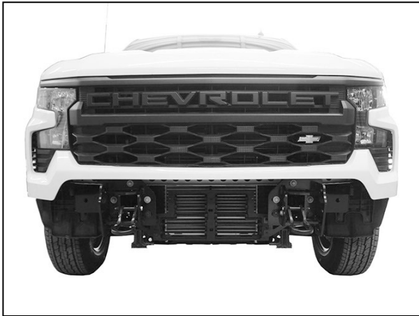
(Fig 18) Reinstall fascia body panel, grille and cover. Reattach inner fender liners
