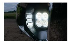
4. Install your assembled bracket and pod onto the vehicle by securing the four original bolts with a 7mm socket and ratchet.
