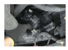
3. Use a 7mm socket and ratchet to remove the four bolts holding the factory fog light housing in place. Remove the factory fog light housing. The factory bolts will be reused.
