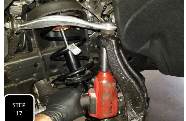
Step 17 Install the new spindle using the factory upper and lower ball joint nuts and tighten. The upper balljoint will get torqued to 60 ft/lbs and the lower ball joint to 100 ft/lbs.
