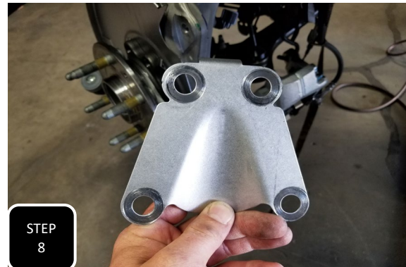
Step 8 Remove the 4 bolts attaching the wheel bearing to the spindle and discard the 4 bolt plate between the bolts and the bearing. NOTE: ONLY 2WD MODELS WILL HAVE THIS PLATE.
