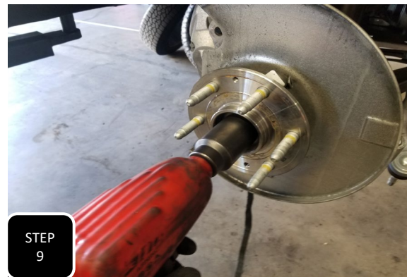
Step 9 On 4wd models you will need to remove the axle retainer nut on the outside of the wheel bearing.
