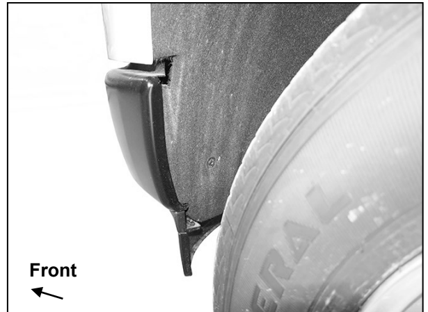
(Fig 2) Remove screws attaching driver/left fender liner to end of bumper
