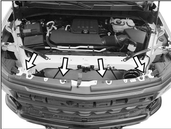
(Fig 6) Remove hardware attaching grille. Firmly pull grille straight out from vehicle
