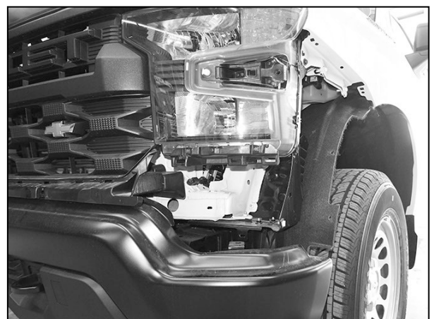
(Fig 4) Remove fascia body panel
