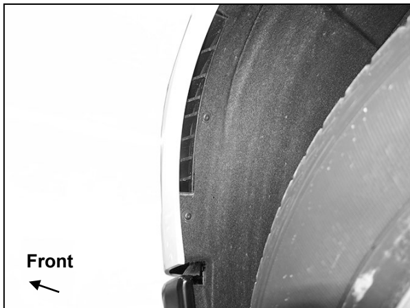
(Fig 1) Remove screws attaching driver/left fender liner to fascia body panel
