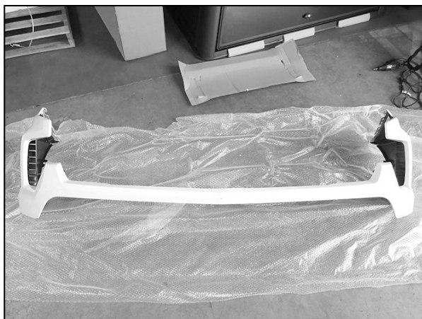
(Fig 19) Place fascia body panel on a clean, soft surface
