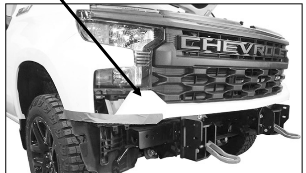
(Fig 23) Test fit Bumper to vehicle and adjust Mounting Bracket locations. Fully tighten Bracket to frame hardware
