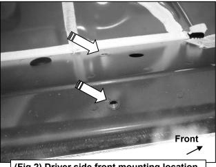
(Fig 2) Driver side front mounting location
