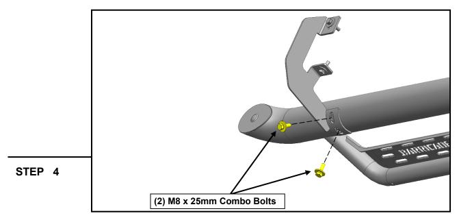
With all brackets loosely mounted to the vehicle, fit the side step onto the brackets, and loosely secure into place using (8) M8 x 25mm combo bolts.
