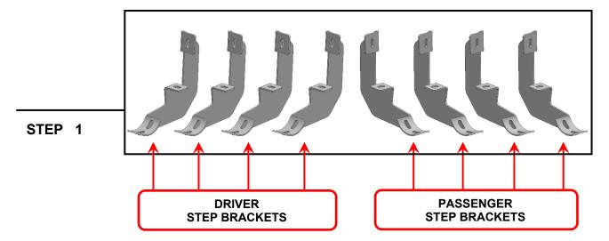
Identify each mounting bracket referencing the diagram above. Notice: The brackets can be used at any position along the same side of the vehicle.
