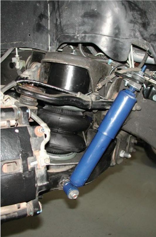
1. The upper shock mount will bolt the rear upper control arm mounting bracket and to the side of the frame rail. It will use one existing hole in the control arm bracket. A 2<sup>nd</sup> 3/8" hole must be drilled in the control arm bracket. A 5/16" hole must be drilled into the frame rail for the 3/8" self tapping bolts.
