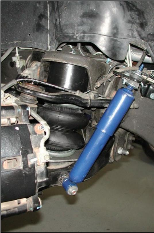
4. Apply thread sealant onto an air fitting and screw it into the top of the air spring.
