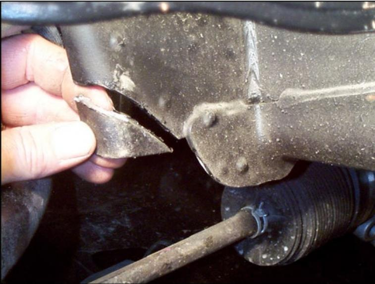
1. The upper coil spring bucket must be trimmed for air spring clearance. The trimmed piece will measure approx. 1 3/4 x 1 3/4. A die grinder and a cutoff wheel will do the job nicely. The objective here is to create clearance for the air spring. Check this area VERY carefully for abrasion against air spring.
