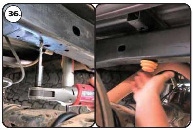
**36.** A hole will need to be drilled and tapped to 3/8"-16 to install the bump stop. This hole needs to located directly above the center of the axle. Mark the location and drill with a 5/16" drill bit. Tap the hole 3/8"-16.. Install the bump stop using a 3/8"-16 x 1" socket head bolt. Hold the bump stop with your hand and insert the bolt through the center of the bump stop. Line up the bolt of the bump with the tapped hole of the frame. Tighten the bolt to 35 in-lbs. Repeat on the other side.
