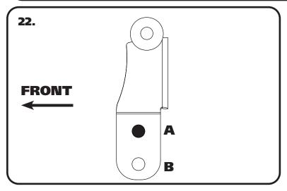
**22.** The rear shackle has 2 leaf spring mounting holes to aid in fine tuning the ride height of your truck. The Standard mounting hole is the top hole "A". Installing the leaf spring in the bottom hole "B" will raise the rear of the truck approximately 3/4". The open side of the shackle will face the front of the truck.
