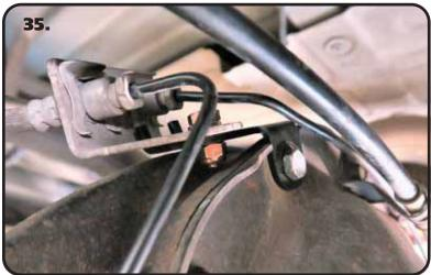
**35.** Remove the OEM brake line bracket that attaches to the differential cover bolt and brake line mount. Attach the new brake line bracket to the differential using the supplied M8-1.25 x 20mm bolt and 5/16" flat washer. Attach the brake line mount to the new brake line tab using (1) 5/16"-18 x 1" bolt, (1) 5/16"-18 nylok nut, and (2) 5/16" flat washers. Torque the M8 to 225 in-lbs and the 5/16" to 17 ftlbs.
