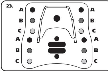
**23.** The hanger can be bolted to the truck at (3) different heights. Position  $A = 5 \frac{1}{2}$ " drop, Position B = 6" drop, Position  $C = 6 \frac{1}{2}$ " drop. If you are unsure where to set it at this time, install the hanger in position A.
