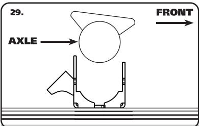
**29.** Set the Flip Bracket onto the leaf spring with the CENTER HOLE OFFSET TO THE FRONT OF THE TRUCK AND THE BRAKE LINE TAB TO THE REAR OF THE TRUCK.
