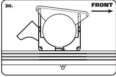
**30.** Slowly lower the axle into the Flip Bracket making sure the tabs go up into the leaf spring saddle. THE FLIP BRACKET WILL POSITION THE PINION AT THE CORRECT ANGLE.
