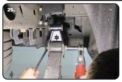
**25.** Install the shackle on the rear eyelet of the leaf spring with the open side facing the front of the truck. Align the top mounting hole with the leaf spring bushing. Install the OEM hardware that was removed earlier. Repeat on the second spring. Do not tighten the hardware at this time.
