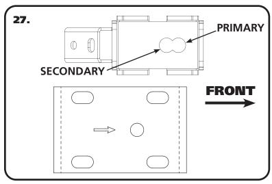
**27.** The Flip Kit has the locating holes offset to center the wheel in the wheel opening. **Image 27** illustrates a top view of the Flip Bracket and the Leaf Spring Plate. The holes are offset to the FRONT of the truck. The Flip Bracket has a brake line tab that will need to be positioned to the rear of the truck. The ARROW in the spring plate should point to the front of the truck.
