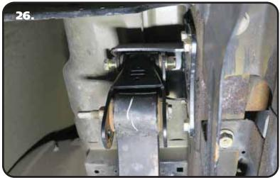
**26.** Raise the rear of the leaf spring up until the rear shackle bushing lines up with the mounting hole of the leaf spring hanger. Install a 9/16" flat washer on a 9-16"-18" x 4 1/2" bolt. Insert the bolt/washer in the aligned hole of the shackle and hanger. Install a 9/16" flat washer and 9/16"-18 nylok nut on the threads of the bolt that are sticking through the hanger. Torque the shackle bolt to 90 ftlbs. The leaf spring bolt will not be tightened until the truck is sitting on the ground.
