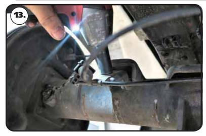
**13.** Remove the bolt from the brake line retainer. The brake line retainer bolts to the bracket that is on the rear side of the leaf spring perch. Remove these from both sides of the axle. These will be reinstalled later.
