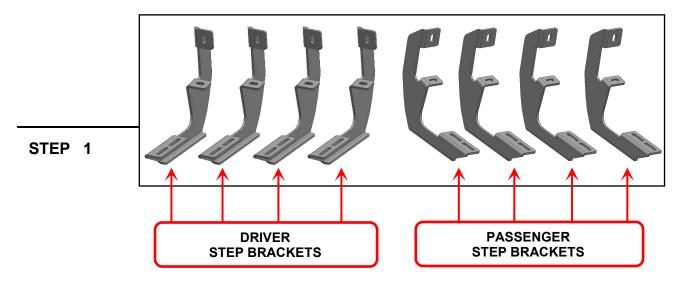
Mounting Brackets are the same. Please identify each mounting bracket using the engraved location identifier. Notice: The brackets can be used at any position of the vehicle.
