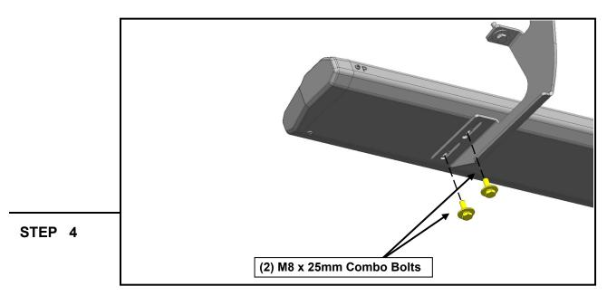
With all brackets loosely mounted to the vehicle, fit the Passenger/Right Running Board onto the brackets, and loosely secure into place using (8) M8 x 25mm combo bolts.
