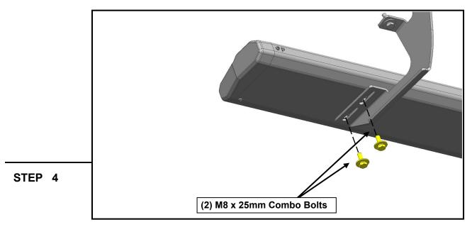
With all brackets loosely mounted to the vehicle, fit the Passenger/Right Running Board onto the brackets, and loosely secure into place using (8) M8 x 25mm combo bolts.
