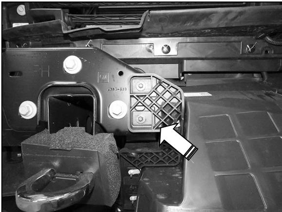
(Fig 3) Remove the bolts and pins attaching the shroud to the vehicle (arrow). Unplug and remove shutter assembly. Driver/left side pictured
