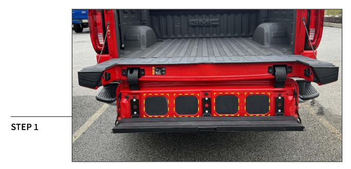
Fold the vehicle tailgate step. Locate the (4) plastic panels in front of the step. Out of the (4) panels, select (2) panels to install the included lights.
