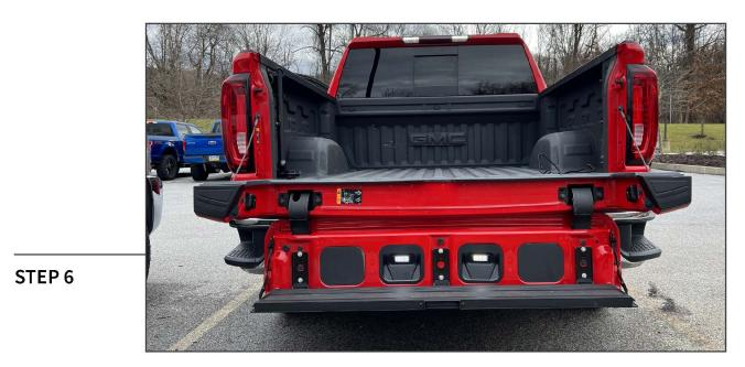
The lighting will power on with the vehicle cargo lamp.
