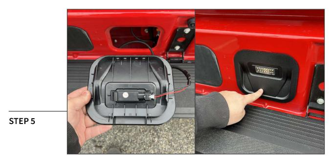
Plug the "T" harness into each LED light assembly, and slide the gray lock to secure the connection. Then, press the LED light assembly into the tailgate.
