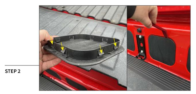
Using a plastic panel removal tool, work the tool around the perimeter of the plastic panels to dislodge the panel from the tailgate.
