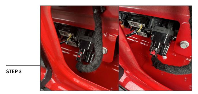
Locate the tailgate latch electrical connector. Slide the red lock down, then press the black tab to unplug the connector from the tailgate latch.
