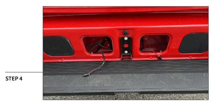
Plug in the included "T" harness in between the tailgate latch harness connector and the vehicle wiring harness. Then, route the LED light harness leads out of the tailgate holes.
