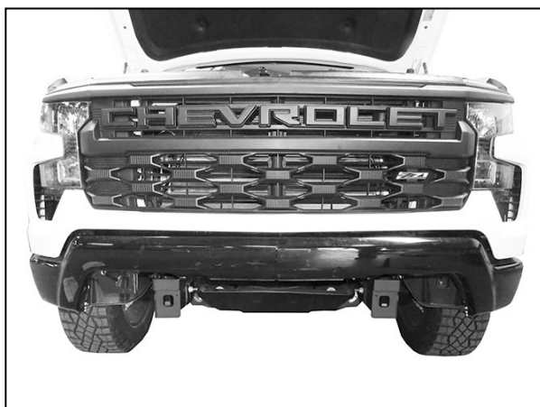
(Fig 22) Test fit CS1 Bumper to vehicle and adjust Mounting Bracket locations. Fully tighten Bracket to frame hardware. Reinstall fascia body panel, grille and cover. Reattach inner fender liners. Models with parking sensors, plug included (2) Wire Harness Extensions into Bumper wire harness. Feed Harnesses out through holes for sensors
