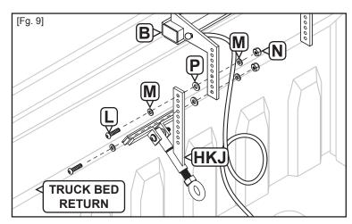
NOTE: Bolts [L] should be placed so that one bolt goes through the top hole of the Cab Support Assembly and the other hole goes through the bottom hole of the bracket located on the Rear Cab Bar.
