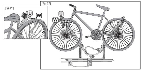
Slide the Lower Wheel Cradle [V] to meet the bottom/side of the bicycle tire.
