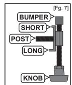
**NOTE:** The Double Bolt Assembly **[D]** provides both vertical and horizontal pressure to fully secure the carrier to the truck bed. If the Double Bolt Assembly is not fully secured or seems loose in either direction (horizontal/vertical) further adjustment/tightening is needed.
